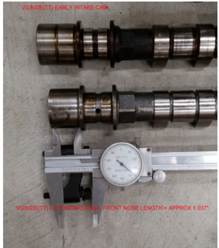
Figure 4 - Late Intake Camshaft Nose Length
