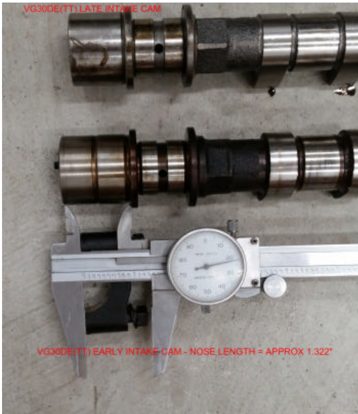
Figure 3 - Early Intake Camshaft Nose Length
